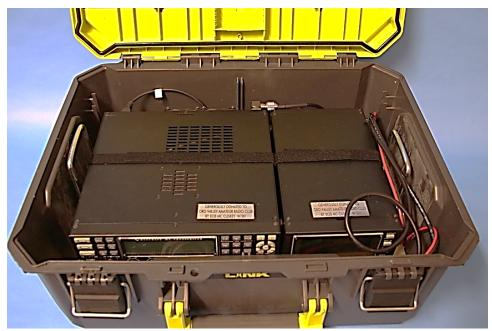
secured and only three cables need to be connected once the Go Kit is deployed. These cables are for the antenna, power supply, and P3 RF sampler.
